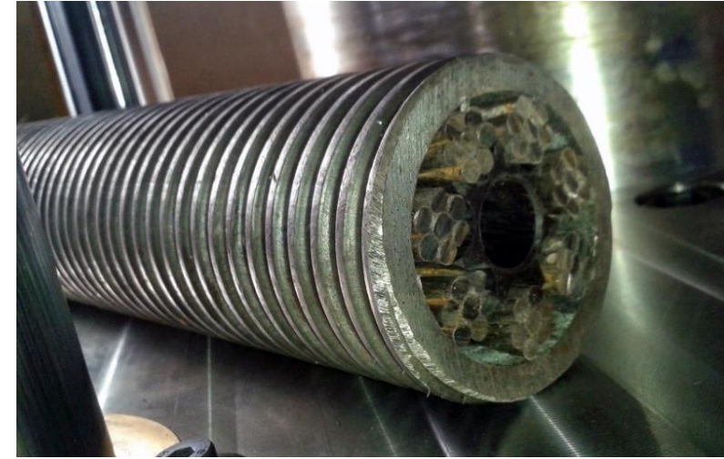
Bar with strands T_{\max} = 3150 \text{ kN}
