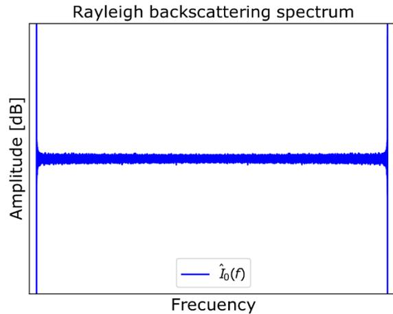
b) By an Inverse Fourier fast transform (Step 1.), the signal is projected in the time domain (distance using the refractive group index).
