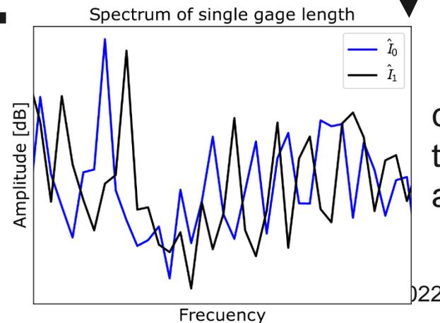
c) The user selects a "window" (gauge length), to which a Fast Fourier Transform (Step 2.) is applied to analyze the frequency content.
