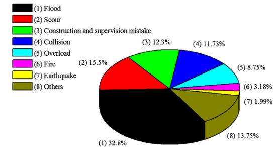
Fig. 2. Distribution of causes of the 503 reported bridge collapses during the period between 1989 and 2000 in the United States (data from Wardhana and Hadipriono 2003)
